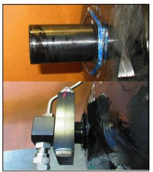
Inspect the slip side cylinder mounting pillow block collar and bushing for any signs of wear or degradation. Any wear or damage that may allow for a cylinder to move more than the specified amount should be addressed immediately.
