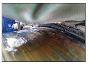
Other indications of heat or fire exposure include burning; charring; discoloration of the coating, label or cylinder; and evidence of connection distortion, such as melted or deformed attachments or installation materials.
