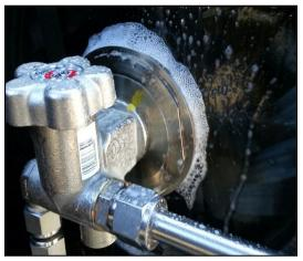
If the cylinder has been in use and has been vented for a service procedure, there will be gas between the liner and the cylinder shell instead of air or purge gases. When the cylinder is pressurized after repairs, whatever gases are present will be expelled; it is not uncommon to trigger a gas detector under these conditions.
