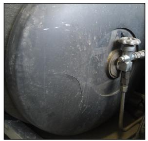
impact damage would be concealed by the dome. In addition to the impact damage, there is also a concern of contaminant intrusion beneath the dome. If the outer covering of the dome is damaged this would allow for contaminants to be introduced and held between the cylinder and the dome.
